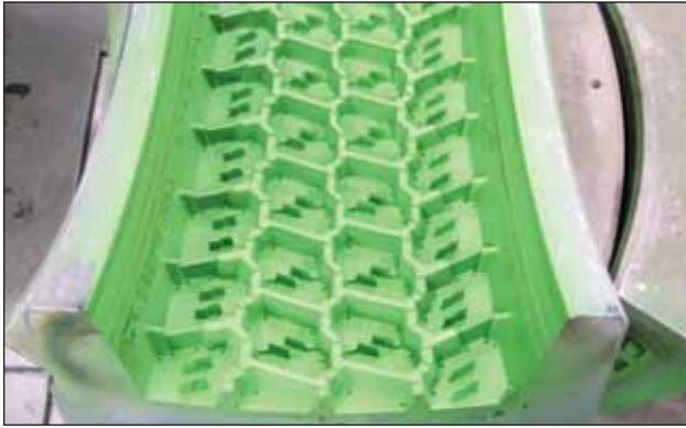
Teflon coating of matrix is a part of the molding system that also includes teflon coating of all bead and sidewall rings.
