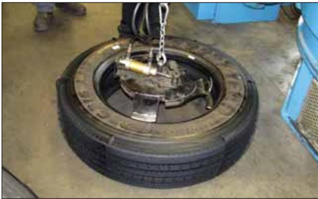
Finished rib design tread is removed from mold.
