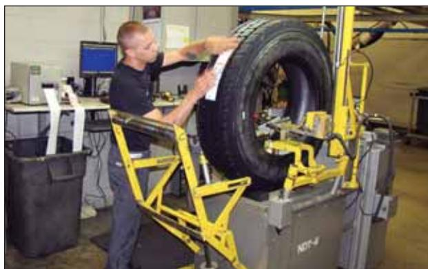
The finished retread is inspected and labeled as part of the final inspection.
