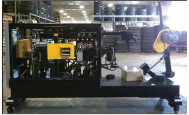
A nearly finished AcuTread 2001 builder on wheels to allow for movement to the building area for testing.
