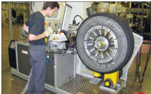
The AZ cushion extruder fills buzzouts and places a thin layer of natural rubber on the buffed surface.
