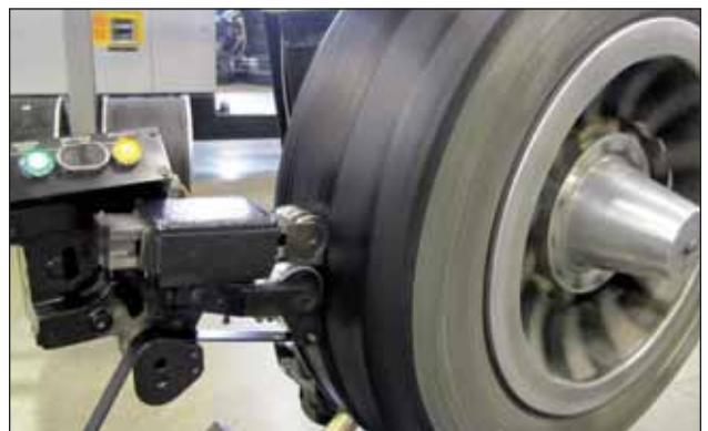
This custom built pin barrel extruder allows high quality, high Mooney rubber compounds to be applied to the tire casing.
